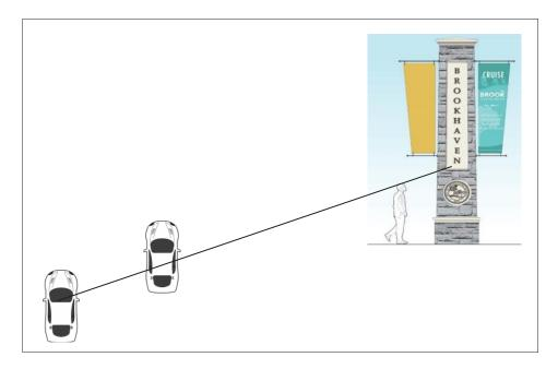
**Figure 4** / Line of sight from observer driver's eyes over blocking vehicle to the bottom of the sign copy.
