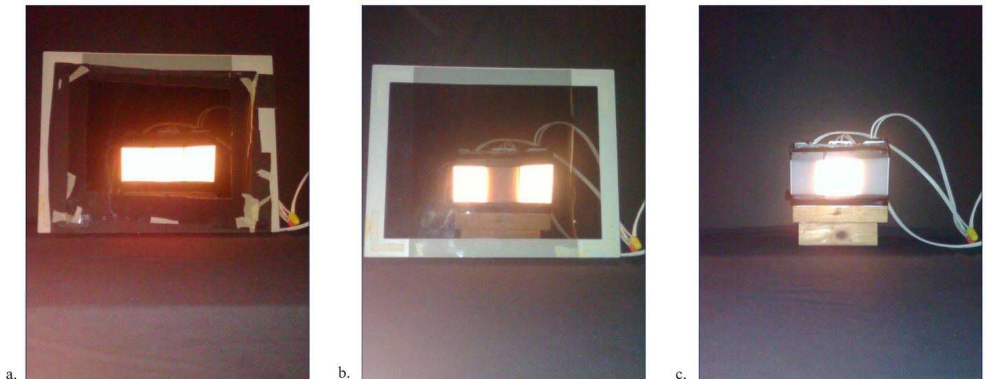
**Figure 2** / a: Display with all panels at 333 cd/m<sup>2</sup>. b: Display with outer panels at 500 cd/m<sup>2</sup>. c: Display with center panel at 1000 cd/m<sup>2</sup>.
