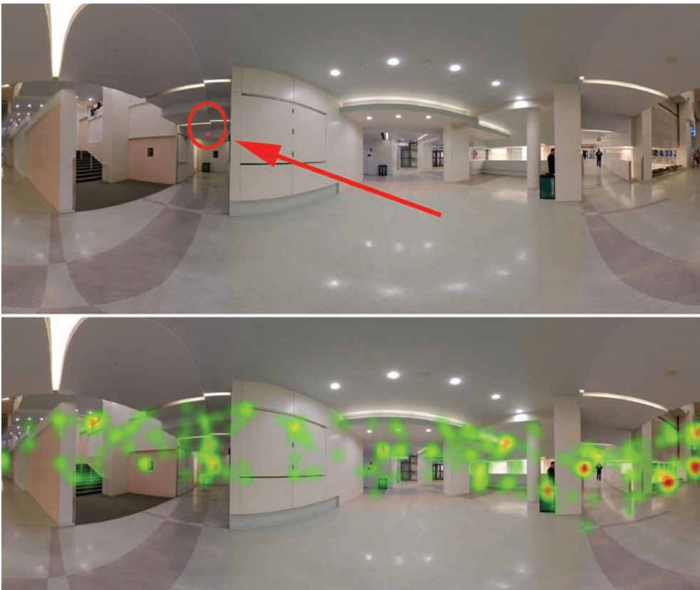
Figure 4 / Interior of campus building where “exit” sign is in a pattern-free wall, within the vertical binocular coverage, and reinforced by vanishing point.
