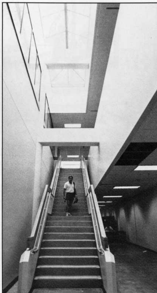
Light wells and skylights keep the center's lower floors in touch with the outside world.
