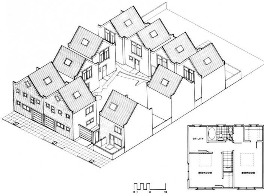
Fig. 5 — 170 Guerrero Street in San Francisco is a typical 10-unit complex of detached affordable housing. The courtyard, shown in the exterior photograph at top, is used for automobiles and pedestrians alike, thus combining functions to reduce costs. The layout of the project and a typical floor plan is illustrated below.
