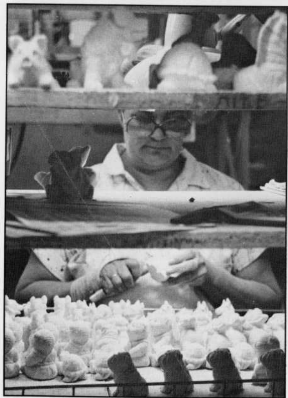
In the fettling area at the Noble plant, a trayful of hydrostone dogs, bunnies and teddy bears await a check for air bubbles and any other imperfections.
