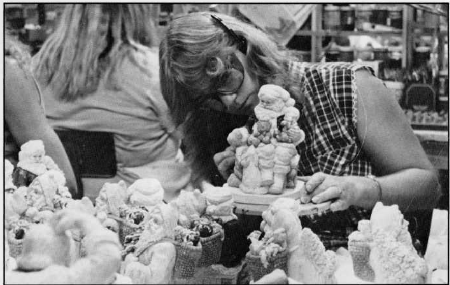
In the production department in Noble, a limited-edition Santa Claus is set on a turntable for easy handling as red paint is painstakingly added to his suit.
