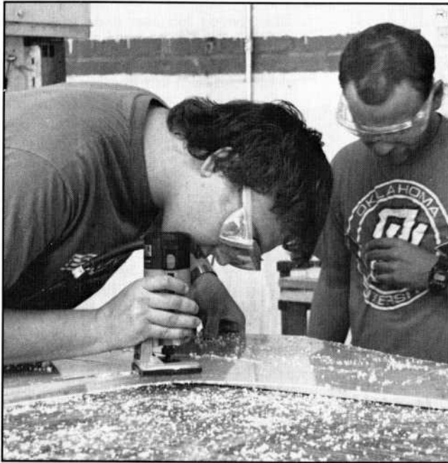
Engineering team members Mark Arens, left, and Richard Liles cut the plastic pieces to be heat formed into the windshield of the OU solar car, The Spirit of Oklahoma .
