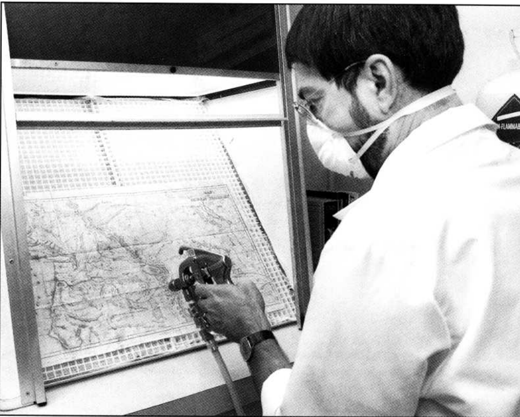
Preserving documents in danger of deterioration is the job of the collections’ assistant curator Bradford Koplowitz, shown here deacidifying a rare map using the Wei T’o Soft Spray system. The WHC preservation laboratory is one of only three such facilities in the state.
