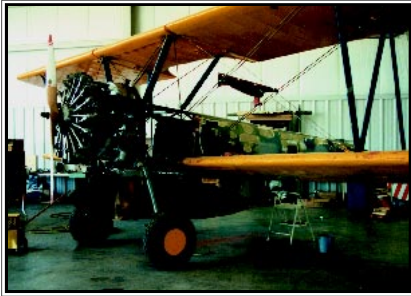
In the Westheimer Field hangar owned by a flight sponsor, his former employer, Harold Powell, Robert Ragozzino's Stearman biplane undergoes its initial disassembly and the fitting of a 150-gallon fuel tank mockup.
