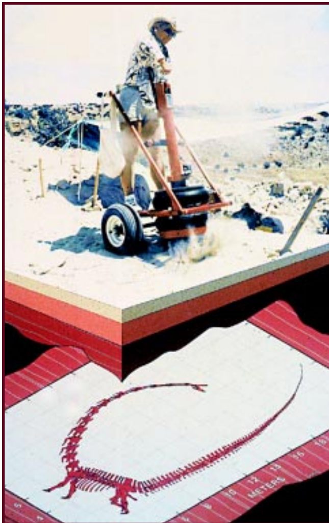
This composite photograph/sketch illustrates use of the seismic gun as the acoustic source to image the buried dinosaur skeleton, Seismosaurus , sketched below in the rigor mortis posture it assumed shortly after death.
