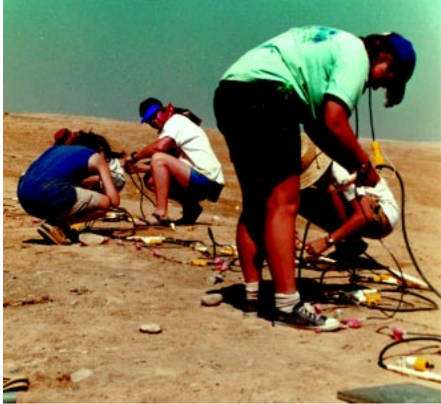
OU's Alan Witten has a toolbox full of geophysical techniques to produce images of objects buried beneath the earth's surface. Students in the photo above are deploying acoustic instruments that can chart the underground tunnels and rooms of a subterranean village that existed 6,500 years ago near what is now Shiqmim, Israel.
