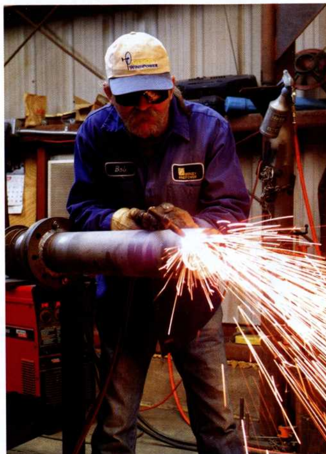
AT LEFT: In the Bergey Windpower machine shop, Doug Sellers checks the micrometer measurements on a faceplate he is finishing for the alternator body. ABOVE: In the welding shop, Bob Fulford cuts the mainframe for the Excel generator.
