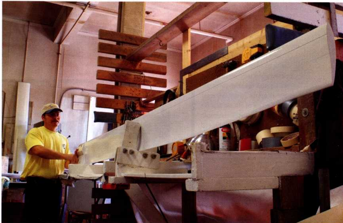
The metal rotor blades on Karl Bergey’s first wind turbines tested well in the laboratory but tended to crack with extended use. Developing a composite of fiberglass and polyvinyl resin solved the problem, and the company replaced all the blades on the old models. Today the blades, here being given a final finish by Ken Parker, are made off-site using the fiberglass “pultrusion” process.
