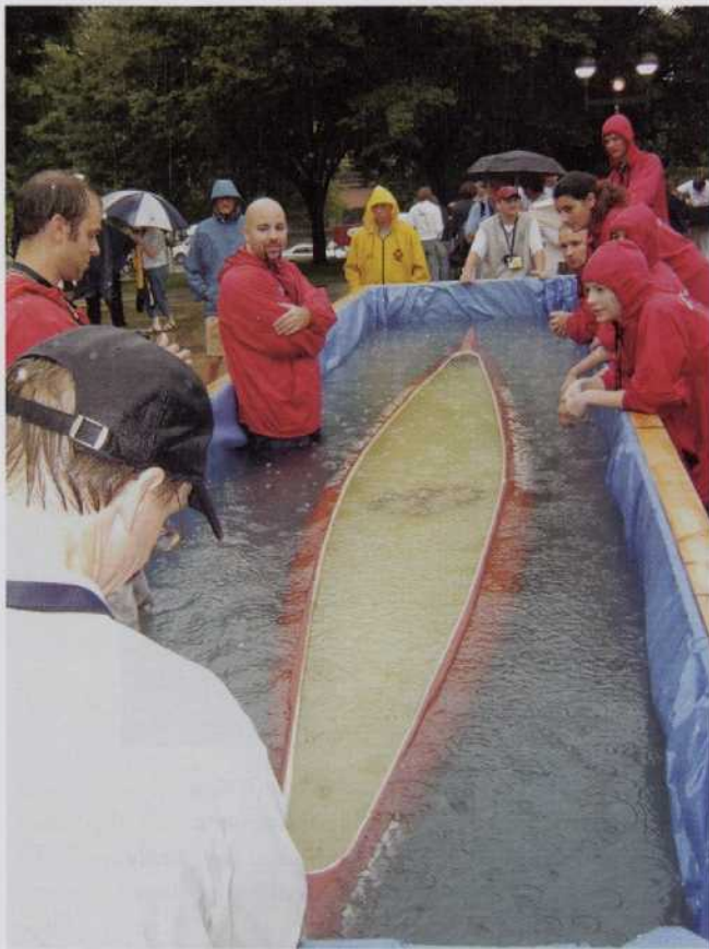
LEFT: All canoes must float, even when submerged in water. Here Kyle LaPointe, left, and Ryan Hague, both standing in the tank, assist a judge, in foreground, during the flotation test in Philadelphia.
