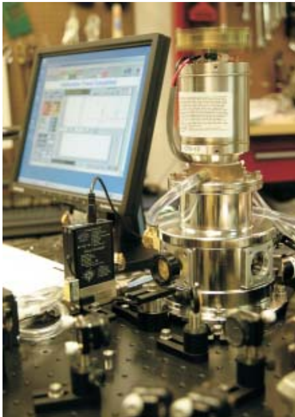
With the Ekids' Breathmeter™ specific molecules in breath samples can be measured for diagnosis and monitoring of diseases such as asthma.
