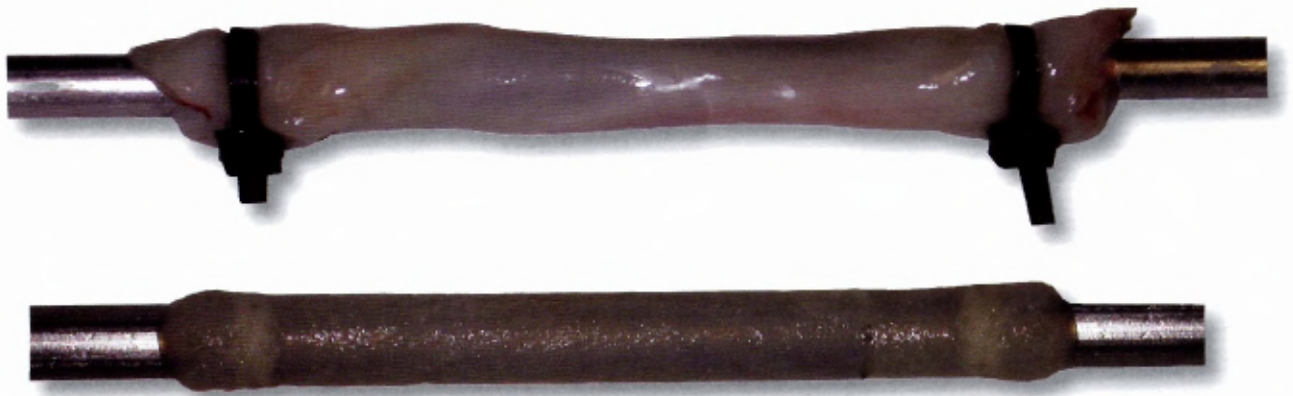
The Human Umbilical Vein (HUV) at top is mounted on the mandrel prior to freezing and machining. The lower image is the HUV immediately after machining and thawing showing a uniform surface structure, cut precisely to a set wall thickness of 0.75 mm.
