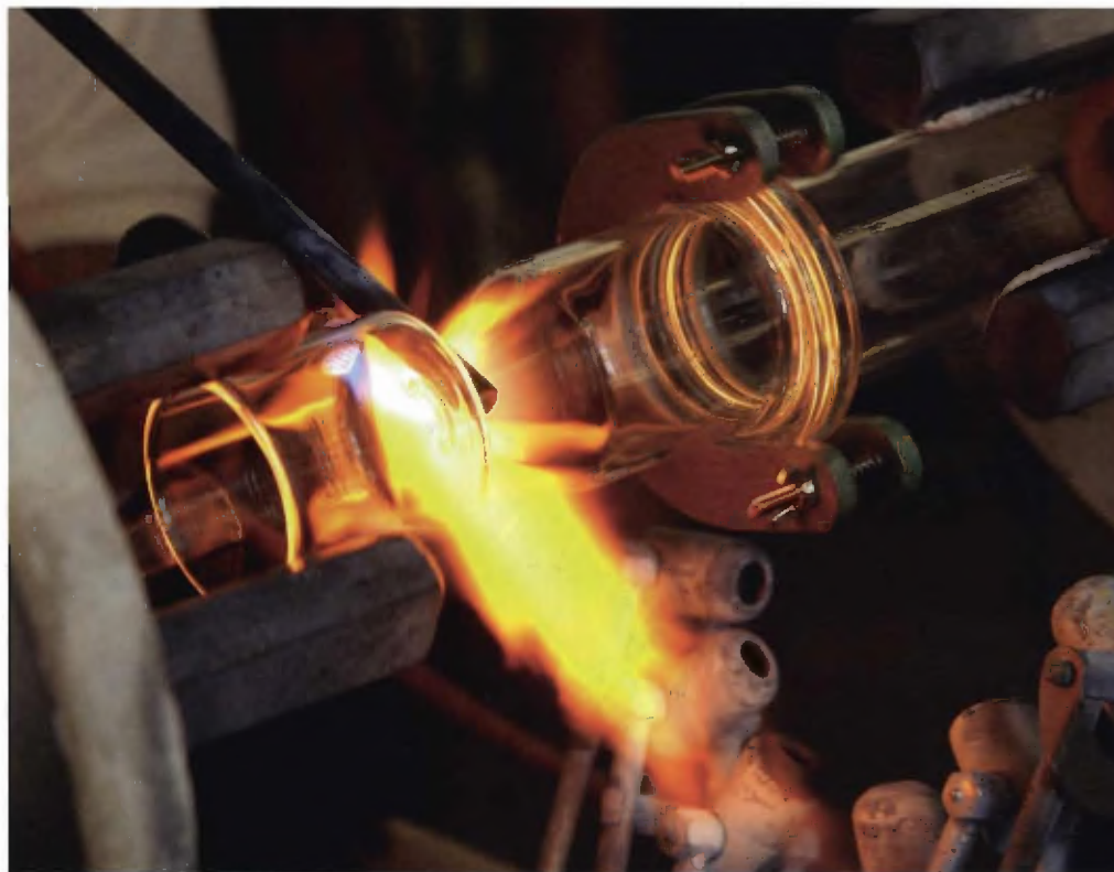
Cornell often uses a lathe to help turn and shape more complex projects. Here, he melts two pieces of glass together to form an hour-glass shaped vessel. The temperature of the liquid glass at the center will climb as high as 2900 degrees Fahrenheit.
