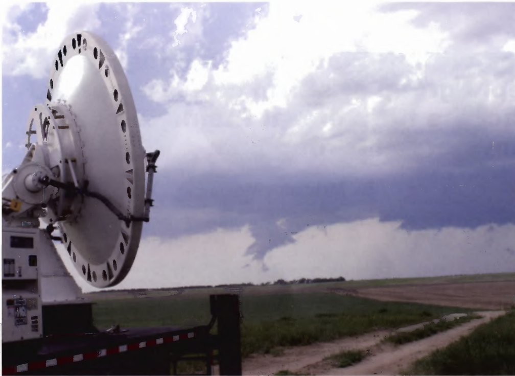
The NOXP radar, jointly operated by NOAA and OU, scans a wall cloud with a lowering a few miles in the distance.
