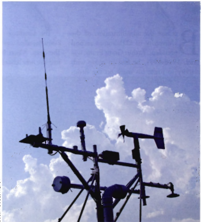
Weather instruments mounted on minivans called mobile mesonets were used to penetrate the storms and measure temperature, pressure, humidity, wind speed and direction during VORTEX2.
