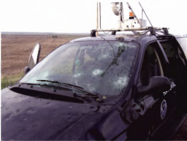
In Wyoming, softball sized hail from the storm that produced VORTEX2's only tornado shattered the windshield of a mobile mesonet.
