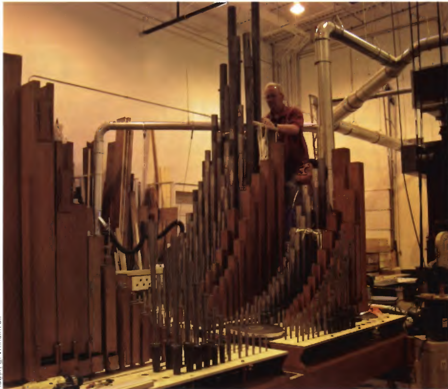
John Goulding, left, and Jeremy Wance install racks for the basses of the main strings. Shorter pipes like those in the foreground require only a lower rack board, but longer pipes need upper racking to provide adequate support.
