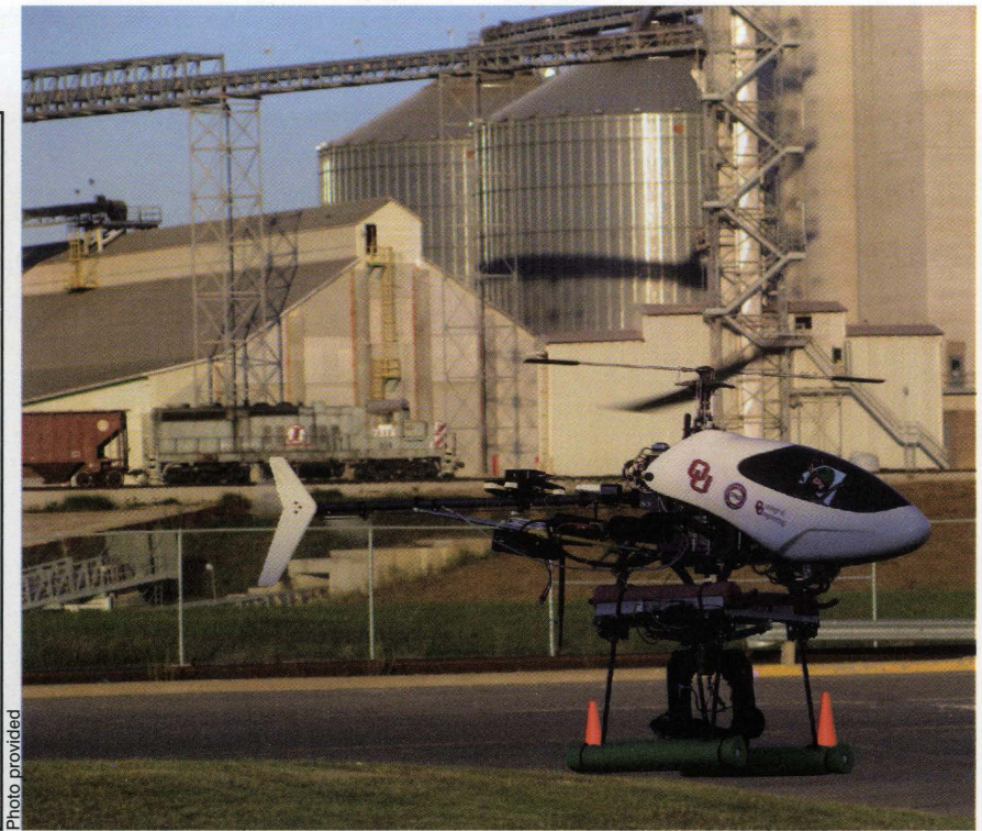
The research team used a building-block approach in creating the $38,000 mini surveillance helicopter, starting with off-the-shelf products and adding other technology.
