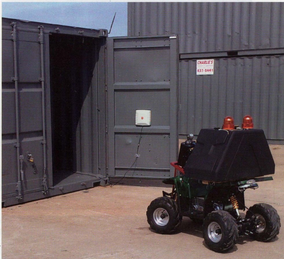
The potential for video surveillance of the vast staging and storage areas at the nation's ports is demonstrated here by the Unmanned Ground Vehicle interrogating an opened shipping container
