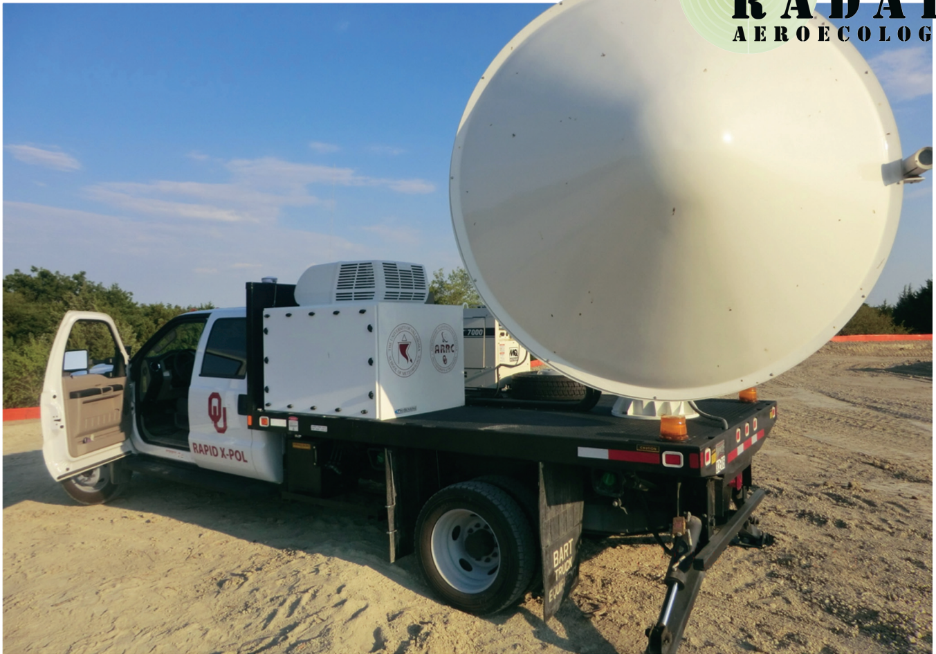
The OU Advanced Radar Research Center's Rapid scan X-band Polarimetric Radar (RAXPOL) has been used to make observations of bird and bat roosts.
