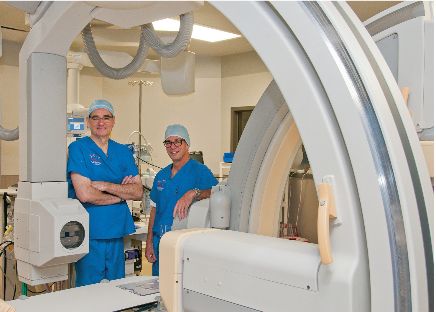
Dyer and Jackman stand next to the fluoroscopy—or live X-ray—equipment. The C-arm can be rotated so that the fluoroscopy is looking through the body at whatever angle is desired. This helps position catheters in the patient's heart. In the lower left is the table that the patient lies on. The table and C-arm are positioned so that the fluoroscopy passes through the chest region.
