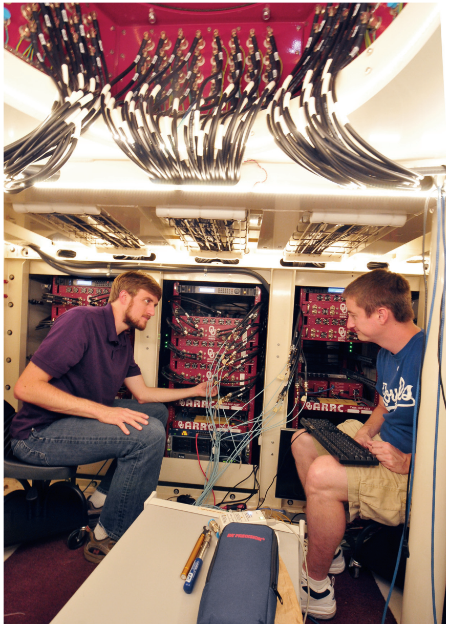
Doctoral graduate students John Meier, left, and David Bodine work inside one of the mobile radar vehicles. This one contains the Cylindrical Polarimetric Phased Array Radar (CPPAR). Built in part by OU students and faculty, there is no other radar like it in the world. The CPPAR can scan a storm rapidly with very high quality polarimetric products, meaning it can distinguish clearly among different types of hydrometeors such as hail, rain, and snow.
