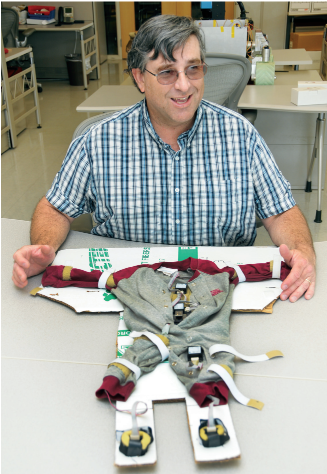
Dr. Andrew Fagg, associate professor of computer science and bio-engineering, explains the robotic “onesie” featuring 12 sensors that gather information 50 times a second from infants as they move.
