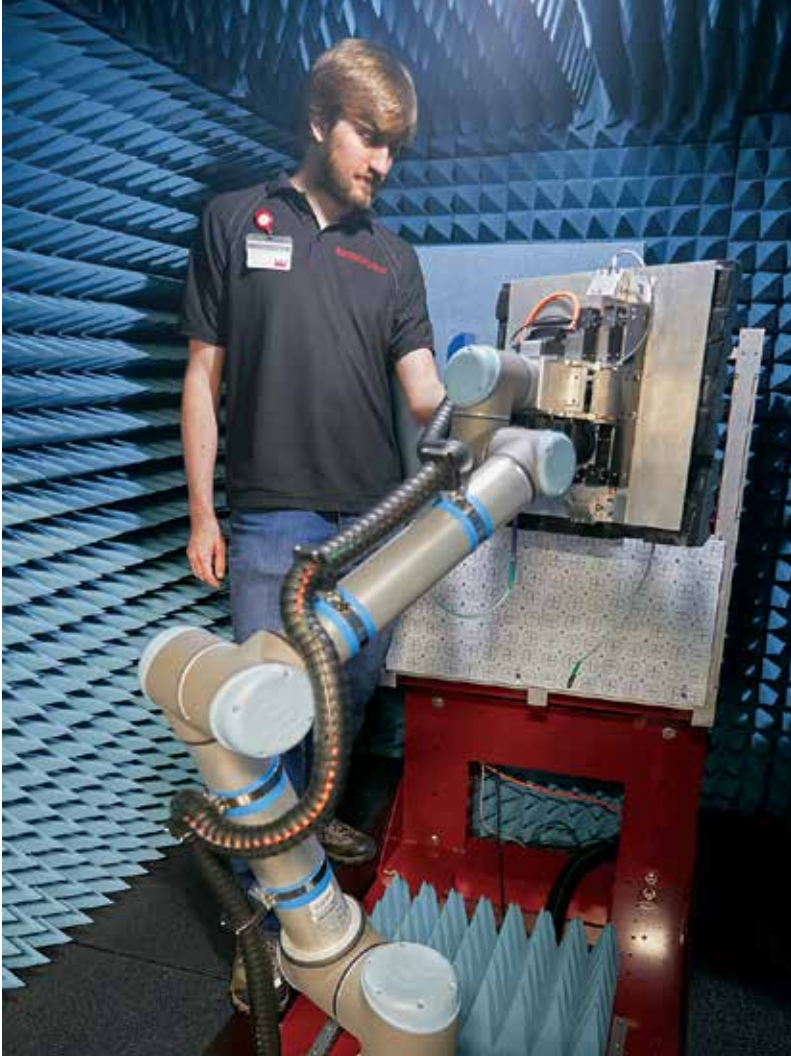
Left - ARRC engineer John Meier uses a robotic arm to test some of the prototype Horus phased-array antennas inside a chamber which controls the temperature and humidity. The blue foam absorbs electromagnetic energy, preventing reflections from interfering in the testing.
