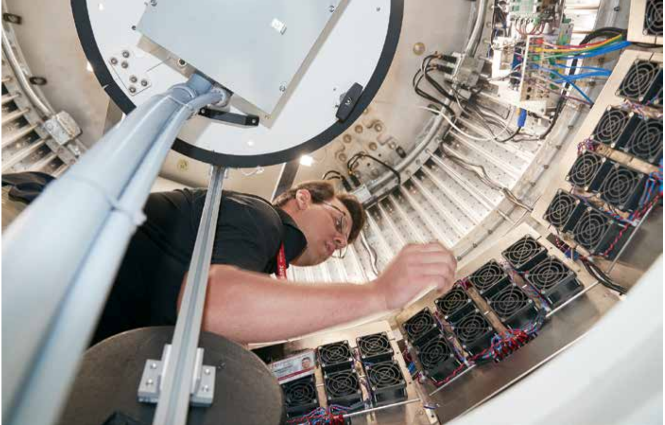
ARRC engineer Matt McCord inspects the connections from the CPPAR electronics to the CPPAR antennas in preparation for transmission from the antenna.
