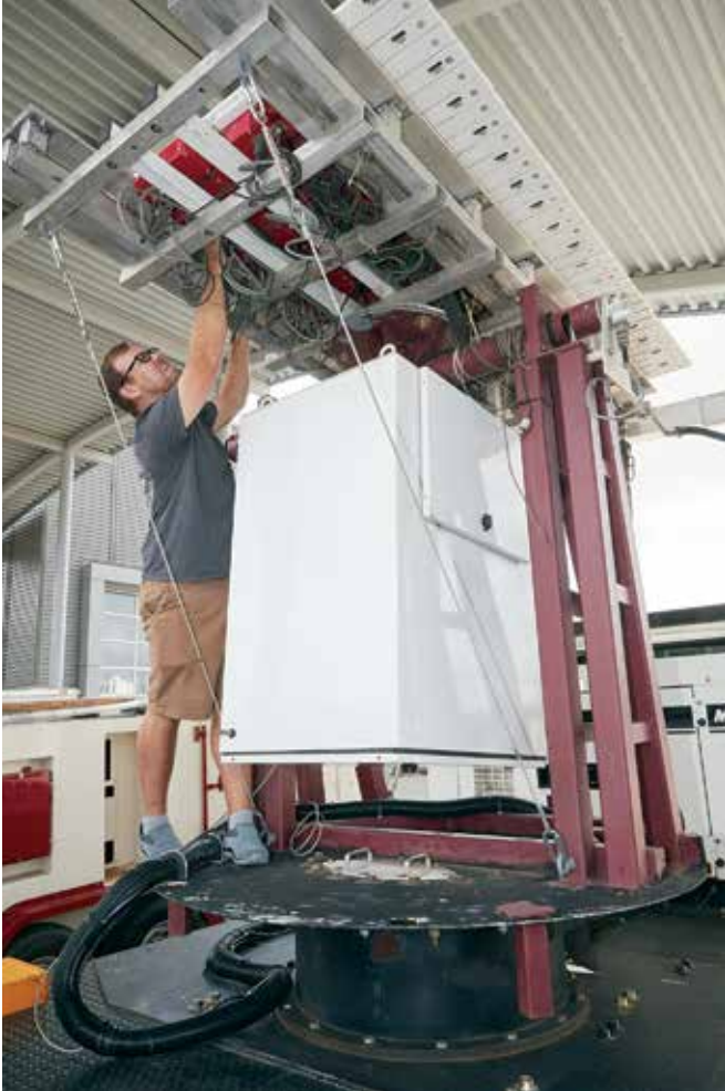
Redmond Kelley, an ARRC staff engineer, checks the radio frequency connections on the phased array antenna for the Atmospheric Imaging Radar (AIR).
