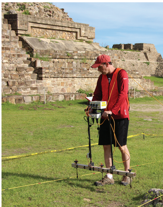
Scott Hammerstedt uses electrical resistance to survey beneath Monte Albán's Main Plaza.
