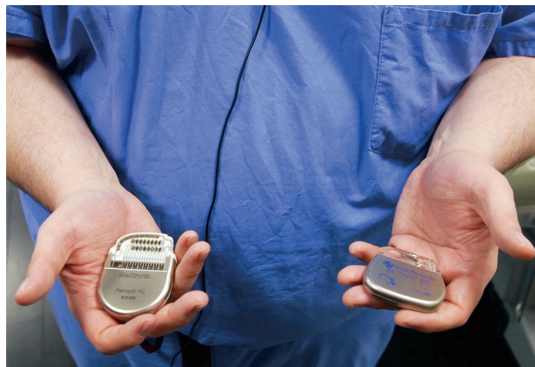
OU Health physicians implant a battery pack under the skin near a patient's collarbone. By occasionally replacing batteries, doctors can extend Deep Brain Stimulation treatments for patients indefinitely.
