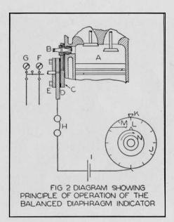
M at the same time in order to complete the electrical circuit and cause a click in the head phones. By taking pressure readings at increment angles through 720 degrees, data is had to construct an indicator card or for other studies.
