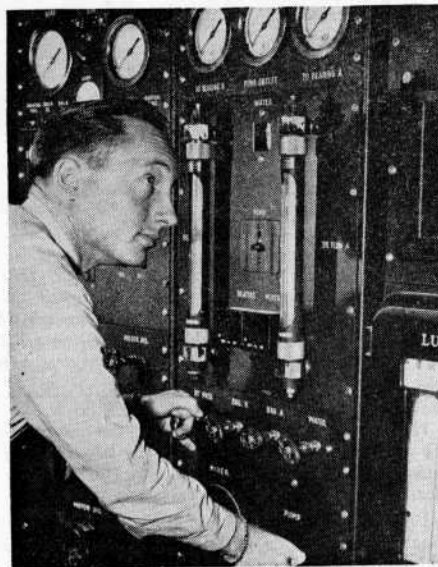
Charles J. Kemp, '42me, is shown here operating the control panel of a machine for high speed tests on ball thrust bearings to be used for gas turbine applications at the Westinghouse Research Laboratories. Kemp recently joined Westinghouse as a member of the graduate student course.
