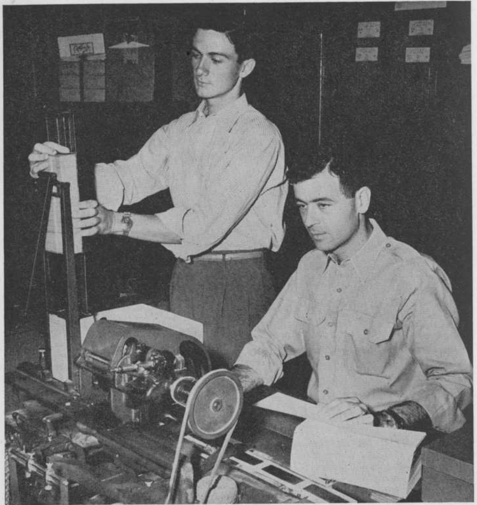
They've got your number. Operator John McGee sits at the addressing machine, stamping your address on slips of paper. The strips are sent to the Press Building, where yours is glued on your copy of Sooner Magazine . Colbert Swanson, assistant address man, feeds stencils into the machine...
