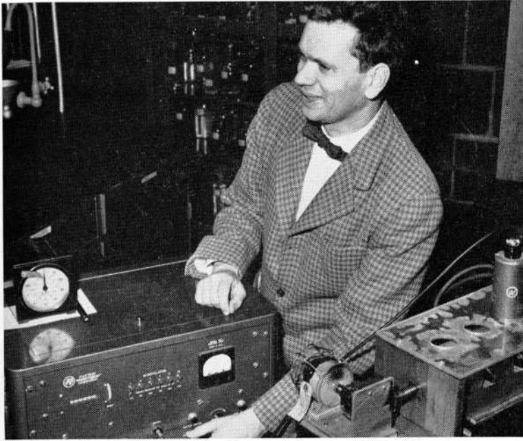
George W. Reid, associate professor of sanitary engineering and public health, is working on the problem of waste disposal. The apparatus at the right is his invention . . . a device to convert sewage wastes into food for fish, animals, by providing the conditions necessary for growth of algae, common fish food.
