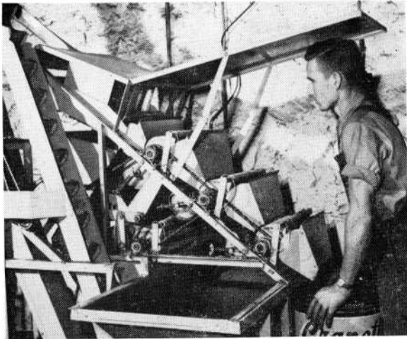
Some nuts are broken during shelling process. Packaged separately from halves, machine gives pieces final cleaning.
