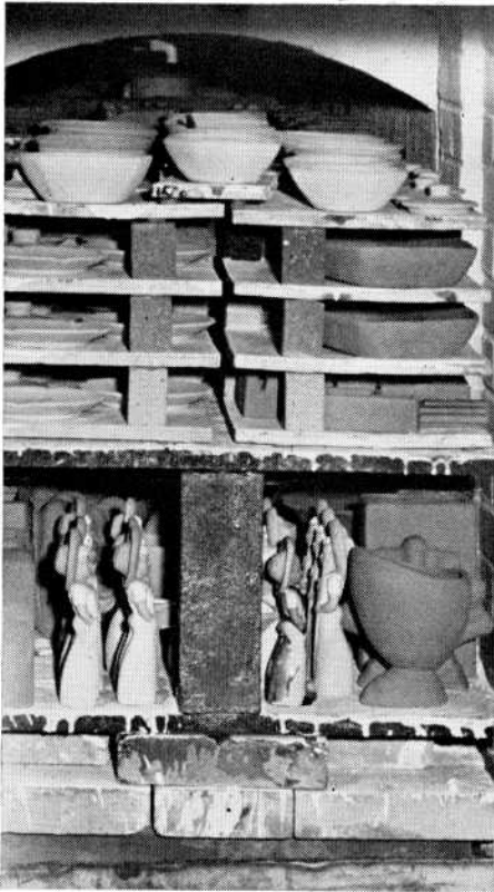
A loaded car enters the kiln to complete Frankoma's unique one-firing pottery process. Standard operation requires firing both before and after glaze is applied, adding to production cost.
