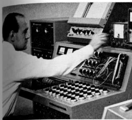
This specially modified analog computer is part of new equipment for process dynamics study.
