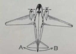
To keep the plane going straight if the engine "X" stops, in which direction should the rudder be moved?
