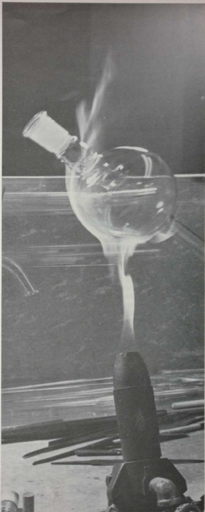
After sealing the internal tube in the flask, Alexandre finishes the job by using a flame to temper the glass to render it less brittle.
