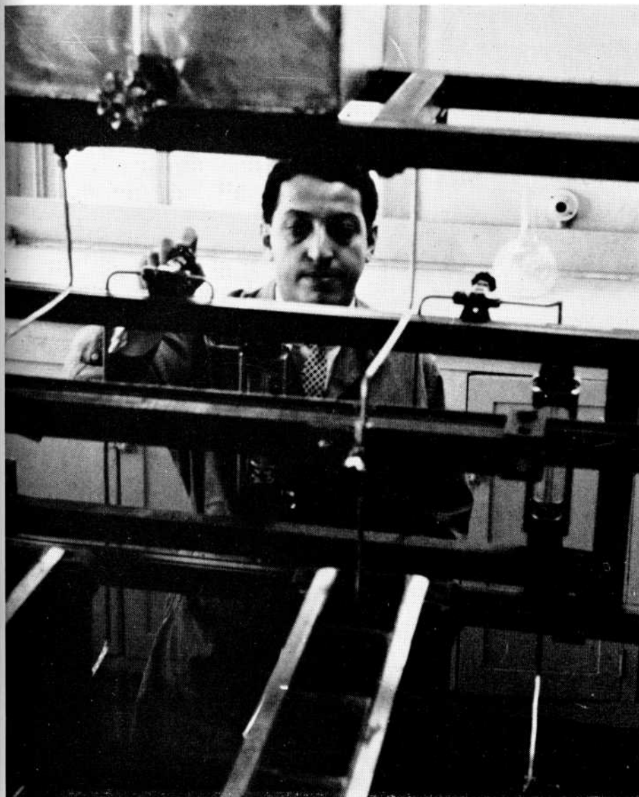
In the laboratory of his New Jersey research and engineering company, Dr. Eldib uses a miniature sewage treatment plant to determine the degree to which wastes can be destroyed by bacteria.
