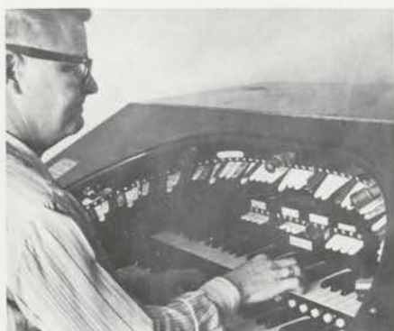
Closeup of Clydes's console. It's a standard Wurlitzer style 210 with nine ranks of pipes and the usual percussions and noise makers.
