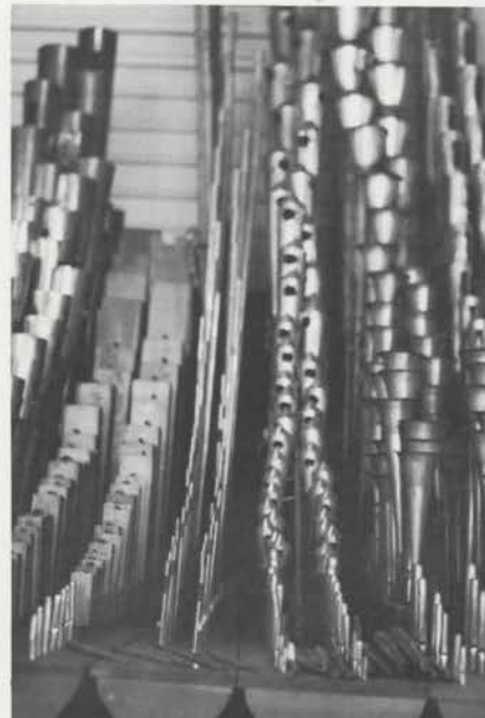
Six rank solo chest as set up in Martin Carport, showing Harmonic Tuba, Gross Flute, Major Violin, English Horn, French Trumpet, and Contra Fagotta.
