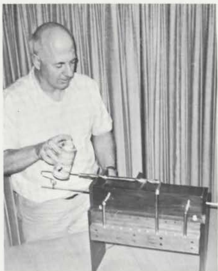
Harvey Heck, researcher in weird and different pipe organ effects, puts the finishing touches on another "positive." He has just mounted the slide whistle. Other noisemakers await mounting.
