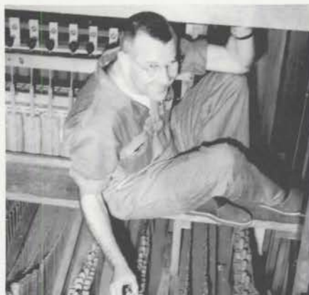
IMPISH PAUL BIRK perches on a catwalk above Choir Chamber pipework to touch up tuning on the Doppelflute. Ranks shown (left to right): Cornet, Doppelflute, Quintadena and Flute.
