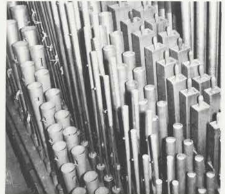
SOLO CHAMBER ranks include (l. to r.): Tuba Mirabilis, Orch. Oboe, Stentorphone (metal flute), Philomela (stopped pipes) and a Gross Gamba are in left chamber, above and behind the powerful and unenclosed Great.
