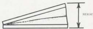
A. THE HEIGHT of the fully-extended pneumatic determines the width of the new material.
