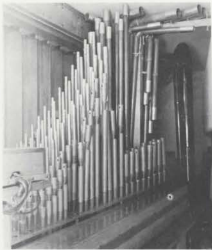
ANOTHER VIEW of the left-hand "Echo" chamber, showing the medium-scale Vox Humana. All three ranks in this chamber are at 8' pitch; all Echo ranks are played from top manual, but may be coupled down. Both Echo chambers are controlled by one swell-shoe.
