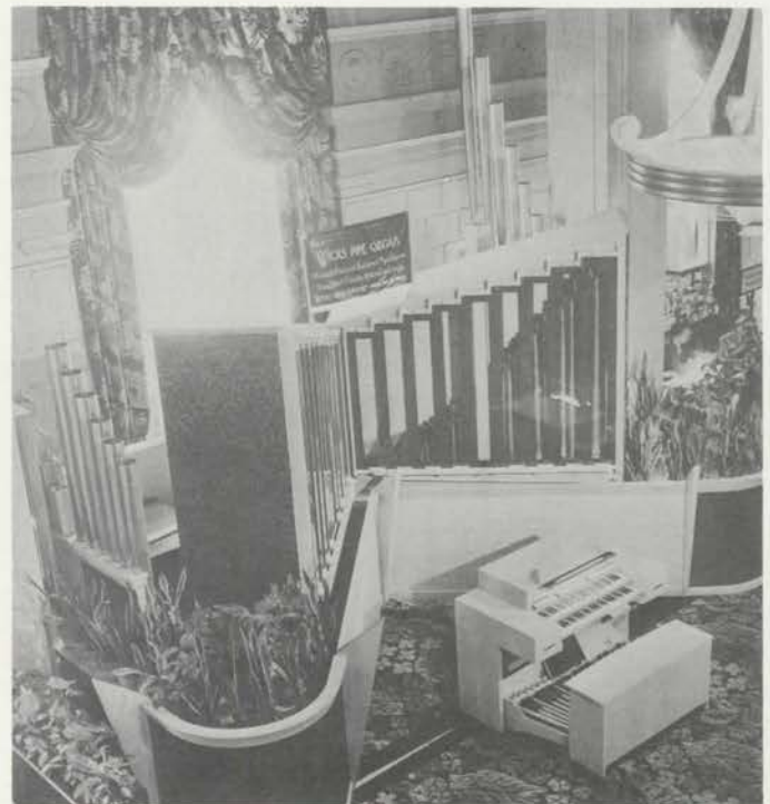
A home-size Wicks built for an exhibition. Note how shallow the swell boxes may be if the large bass pipes are left outside. At the left can be seen six of the 8' Open Diapason pipes and part of the 16' Bourdon. Behind the right swell box are the 16' Trombone pipes. These would be mitered for a normal low-ceiling home installation. The conical pipes in the right swell box belong to the Gemshorn, a member of the Diapason family.
