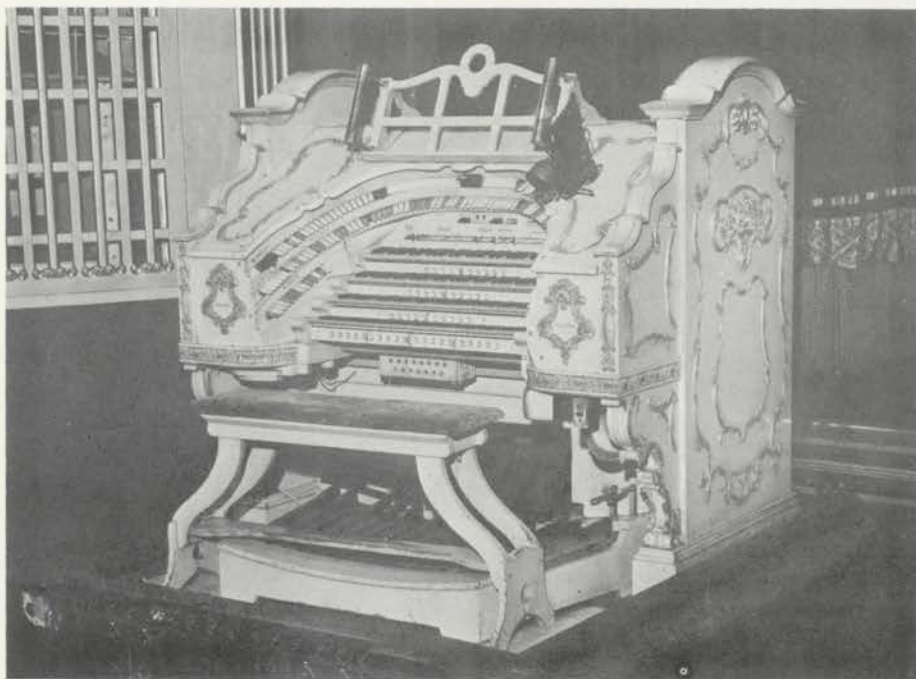
Opus No. 2170, a French design console, was shipped to the Odeon (Paramount) Theatre in Manchester, England, on 7/14/30. Clearly visible are the six stops added as a second row of tablets. The four black couplers were moved up from the bottom row, and the Vibraharp and Vibraharp Dampers stops were an added feature on the later issues of the Style 270.
