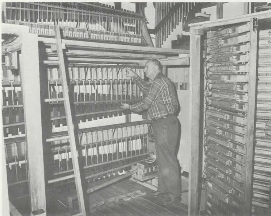
Edwin A. Link adjusts the marimba-harp stroke in Roberson Center organ. Switch and relay stacks at right.
