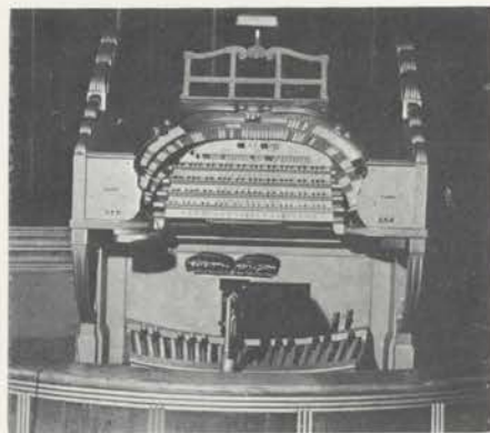
(Above) Opus No. 2170, Manchester, England, showing stop tablet layout. Note non-standard engraving on the stop tablets.
