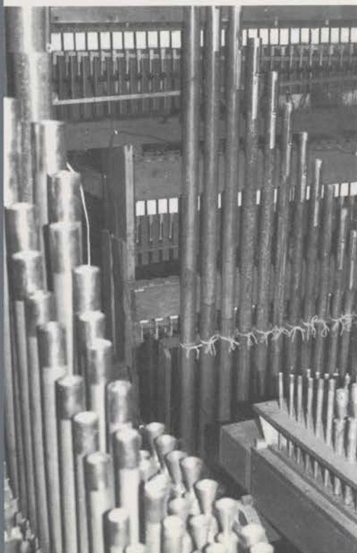
Partial view of pipe chamber showing Tibia, Diapason and Kinura ranks in left foreground. Tuba chest right foreground. String offset to rear with chimes, orchestra bells and xylophone.
