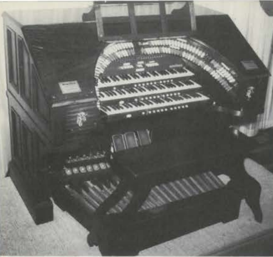
The CIPHER HILL console. When Dean bought the organ, parts of the console were missing, including swell shoes and crescendo pedal. They were replaced by shoes from an Allen electronic. — (Floyd Tillman Photo)
