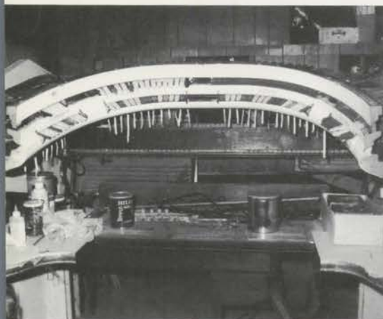
Console during process of re-installing stop tablets — pneumatics have been releathered.
