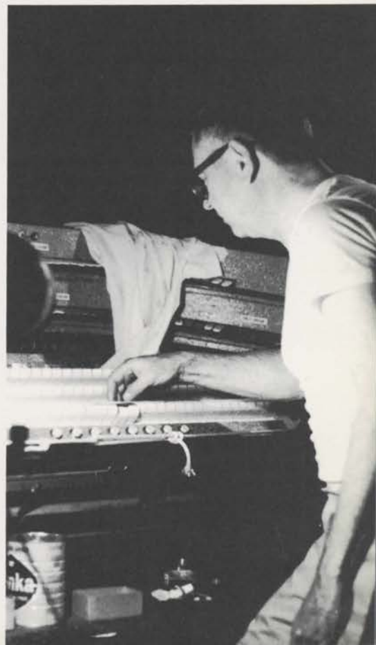
Ben Levy, Motor City member, adjusts second touch springs on the 3/13 Barton.
