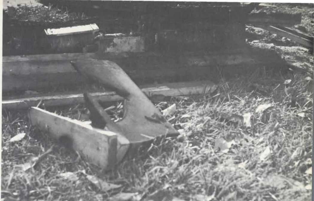
All that remains of the console. Note the two large coils in the upper left. These were holding coils of the Austin capture action.
